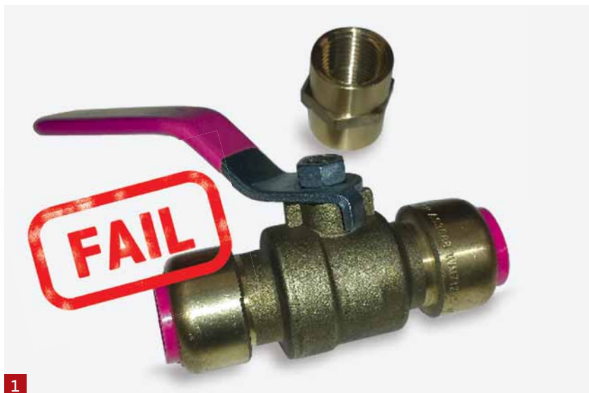
1 IMAGE 1: Both products failed to meet DR requirements and could more than likely fail before their expected usable life is over. IMAGE 2 & 3: Dezincification test results indicate both products do not comply with product standards.
