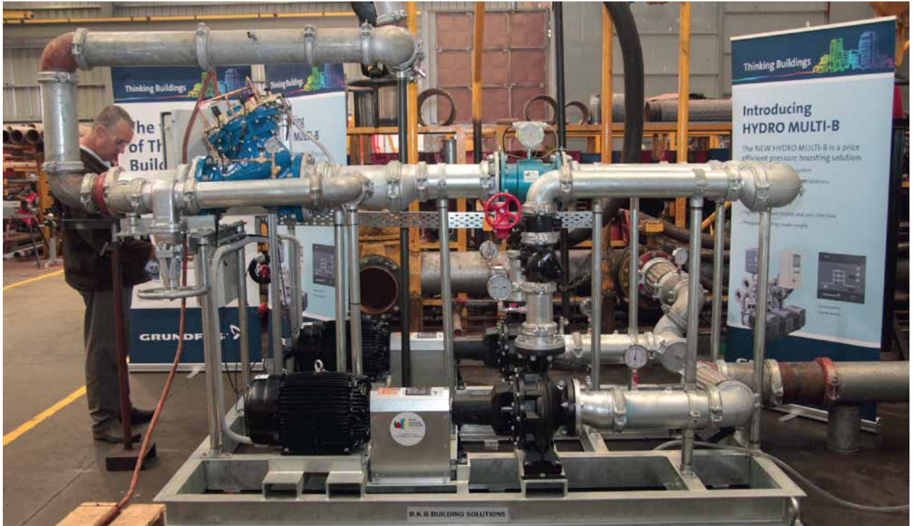
The dual pump system, developed by BKB Grundfos sees both pumps able to simulate up to 50L/s.
