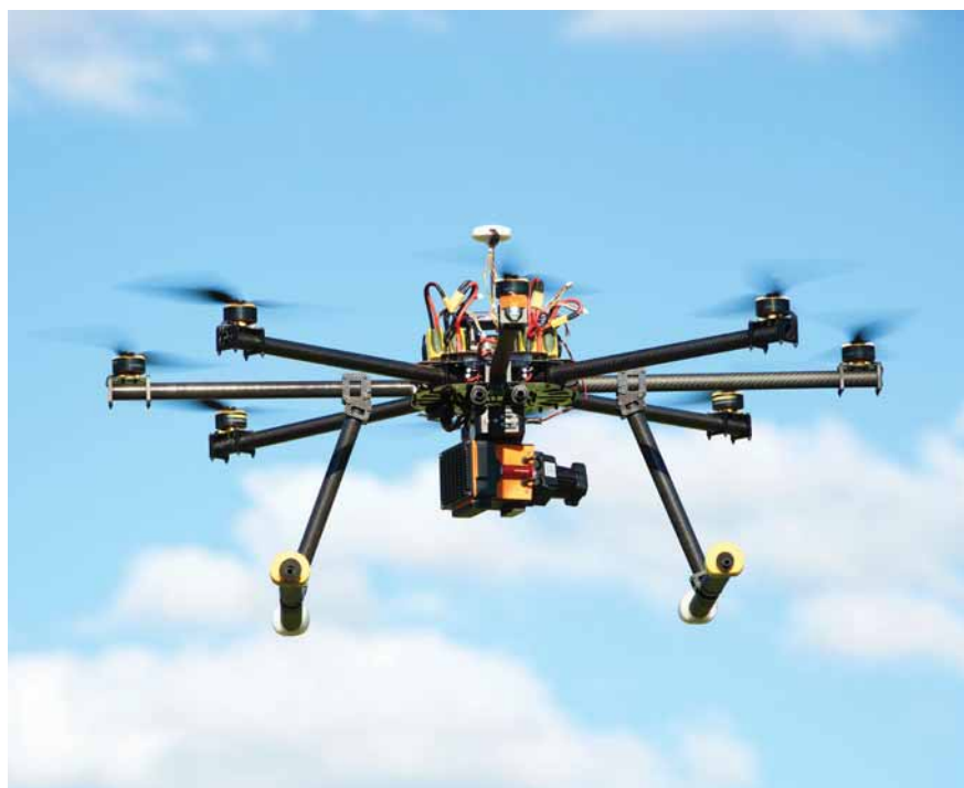
The CSIRO has developed a 3D LiDAR payload that can simultaneously map its surroundings while sensing its position in the 3D space.
