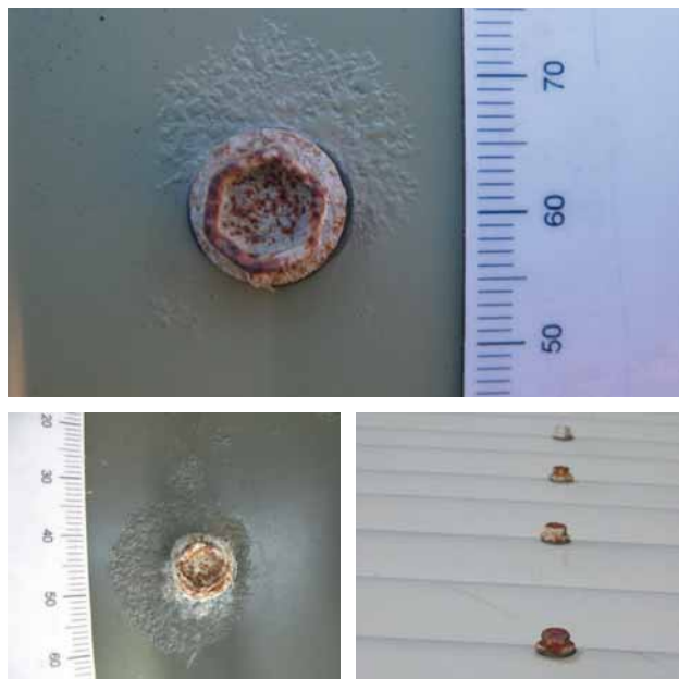
Metal roof screws are the first parts to fail if the products' corrosion resistance coating is not fit for purpose.
