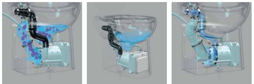
The Sanicompact C43s flushing, macerating and pumping processes takes around 10-15 seconds from start to finish.
