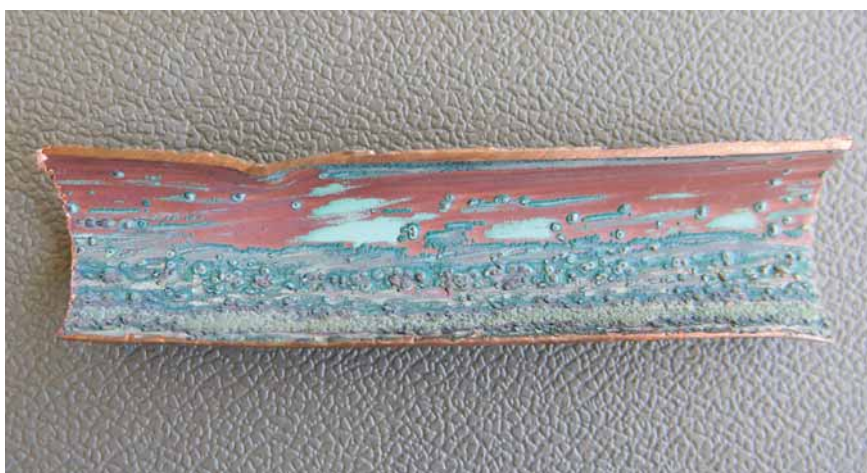
If PPR pipe fails, it generally occurs in the same location within the building, depending on which multiple simultaneous factors it was exposed to. In my experience it is typically a very small percentage of the total amount of pipe that is affected. This image is of a transition between a totally oxidised pipe to further down the line where the majority of the pipe was undamaged. Different factors are more prevalent in different parts of the system. The key is knowing how to turn them off.
