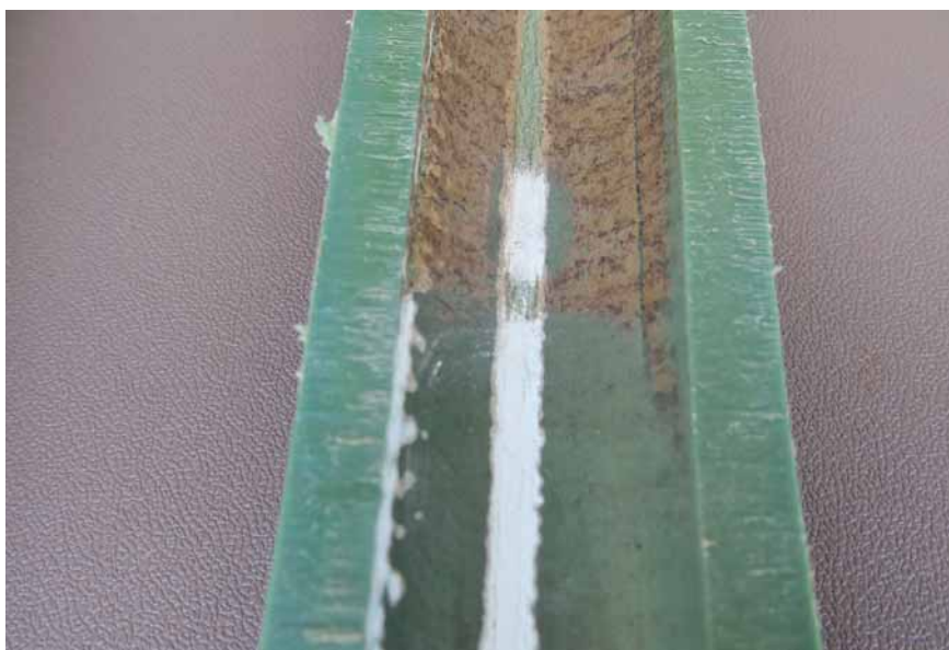
This copper pipe was installed in an area where there were very high free chlorine levels. It was interesting how the pipe damage changed dramatically depending on the orientation of the pipe. This indicated that chlorine on its own was not the only contributor.
