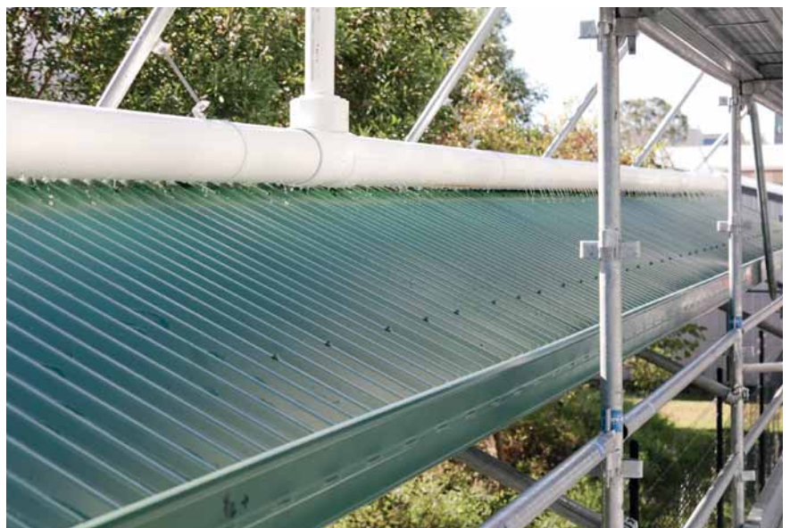
Residential Roof Drainage Test Rig developed by AHSCA and SWRG, University of the Sunshine Coast
