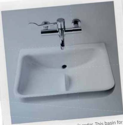
Infection control is on everyone's radar. This basin for medical facilities features a built-in hydrofoam, which resembles an upside-down winged keel, to reduce splash and the accidental spread of infection.
