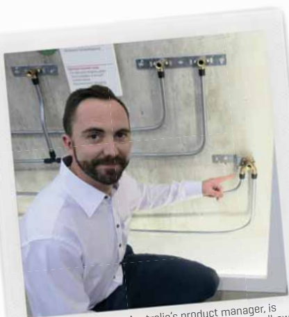
David Cole, Rehau Australia's product manager, is enthusiastic about this new U-shaped wall plate elbow which enables continuous water flow to the tap, to eliminate dead legs on hot water lines, thereby reducing the risk of bacterial growth in potable water lines.
